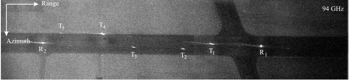
Fig. 4. 94 GHz focused SAR image recorded simultaneously to the one in (Fig. 3). Note how the moving targets are misplaced differently here than at 35 GHz because of different Doppler shifts.
