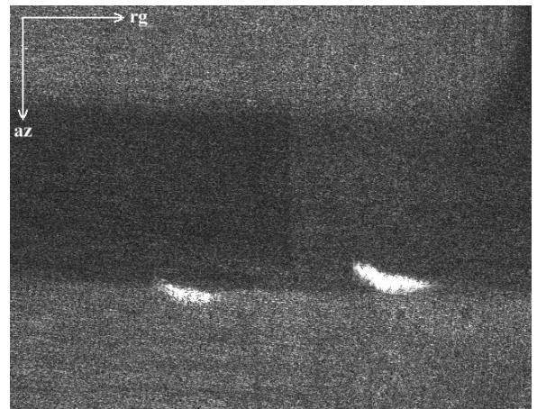
Figure 6: 35 GHz SAR image of two Puch multi-purpose vehicles moving on a road at 15 m/s in positive range direction. Image resolution is 0.19 m.
